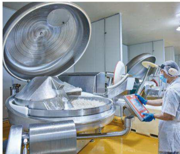
Worker operating bowl cutter with programmable recipe-management system.
